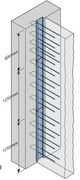
Wall connection using two 1250 mm HBT Elements and a 800 mm HBT Element to obtain 3.30 m floor height
