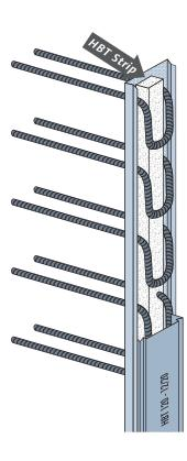
Due to inherent low concrete cover and restriction in element size in precast elements, demands on precise measurement and manufacturing of rebend connections are generally higher.
