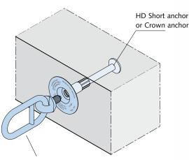
HD Link or ring bolt; is attached during installation as a permanent fixture.
