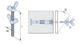
The retaining bolt is used to attach the steel nailing plate. A butterfly bolt is crimped to one end to tighten the bolt; an additional butterfly bolt is used to secure the bolt to the formwork.
