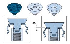
Identification caps are packed separately. These must be fitted to the appropriate HD Anchor which has the same identification colour. The integrated thread protection remains in the HD Anchor permanently (Fig. 4).
