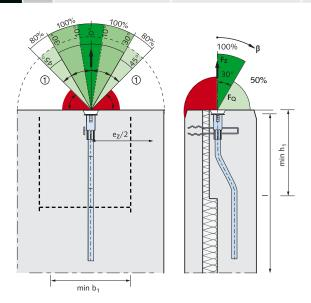
Angle range from 10°: Only permitted with 6367 Rotary head lifting link!
