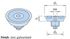
The zinc galvanized steel HD Magnetic plate can be used to secure HD Anchors to steel formwork. Available for thread sizes from Rd 12 to Rd 52. The nailing plate creates a recess in which the perfect-head or the adapter is fixed.
