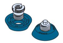
The HD Nailing plate which consists of a steel core and a replacement ring is used for fixing a HD Anchor to the formwork. Available in thread sizes Rd 12 to Rd 64.
