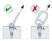
The recess in the concrete made by the nailing plate matches the shape of the HD Lifting links exactly. This allows the lifting link to rest against the concrete when the anchor is subjected to diagonal or shear loads.
