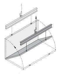
The shear reinforcement on both sides also serves as diagonal load reinforcement. Additional diagonal load reinforcement is not required.
