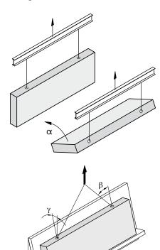
The shear reinforcement can be omitted when using a tilting table and a load angle of  $\gamma$  < 15°.
