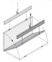
The shear reinforcement on both sides also serves as diagonal load reinforcement. Additional diagonal load reinforcement is not required. The additional shear reinforcement must be installed with full contact to the threaded socket.
