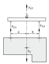
The centre of gravity of the load will always stabilise verticality under the crane hook. Load distribution in nonsymmetrical installed anchors when using a spreader beam is calculated as follows:
