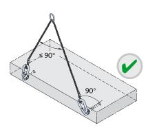
Installation of the HD Lifting System
