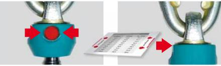
Check the colour security-mark on the plug. The security-mark must not have anv cracks.
