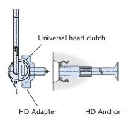
Alternatively, if a spreader beam is not available it is possible to use the rotary head lifting link 6367 or the HD Adapter no. 6366 in combination with the universal head link no. 6102.
