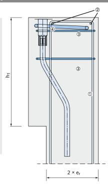
The offset HD Anchor must be completely enveloped in concrete. The thickness in the load-bearing layer needs to be increased around the HD Anchor. The concrete cover on all sides of the anchor must be at least 2.5 cm.
