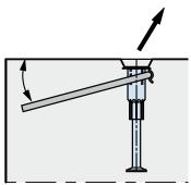
Always install diagonal rebar opposite the direction of the load.
