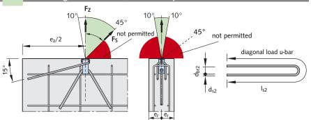
The minimum permitted axial spacing between lifting anchors is  $e_z$ . The required hanger reinforcement is inserted through the lower hole in the HD Plain anchor. The hanger reinforcement must be secured in place with full contact to the anchor. Refer to the reinforcement drawings and tables for each load class for any required additional reinforcement. The value given for concrete strength  $f_{ci}$  is for normal concrete according to DIN EN 206 or DIN 1045-1.
