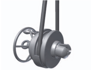
Turn the handwheel to open the clutch.
