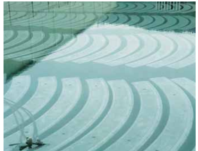
Underwater storage of tubbing segments
