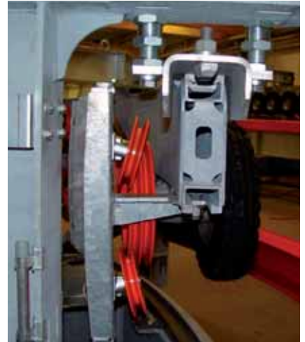
Roller-bearing fixing of a cableway
